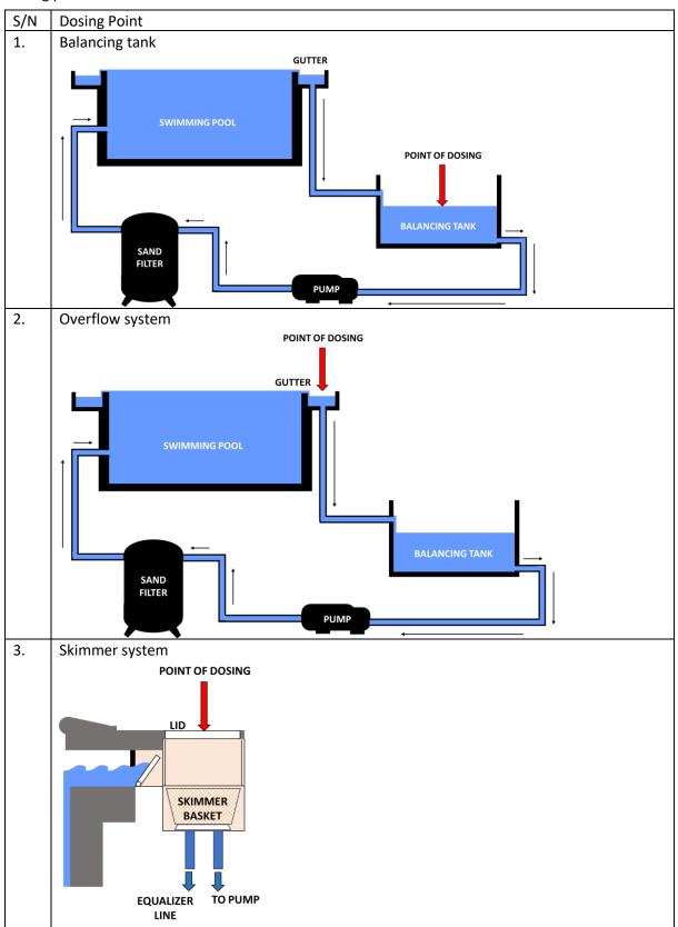
Example of working principle for automatic chemical doser
