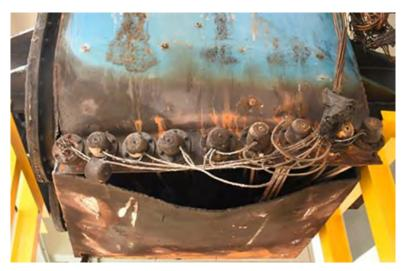
Figure 3. Bottom view of damaged mixer taken by MOM
