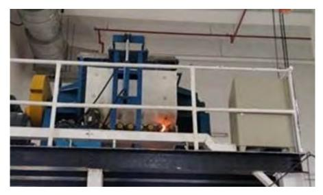
Figure 26. Image showing glowing flange connection of one of the mixer's heating element
