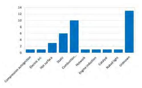
Figure 18. Breakdown of aerosol related incidents according to ignition sources
