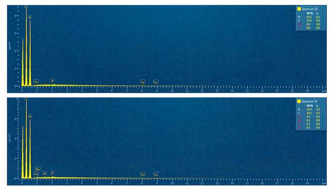
Figure 5c: EDX Spectrums 18 and 19 - Elemental Compositions of "Bulk (Potato Starch), (080321-4b)"
