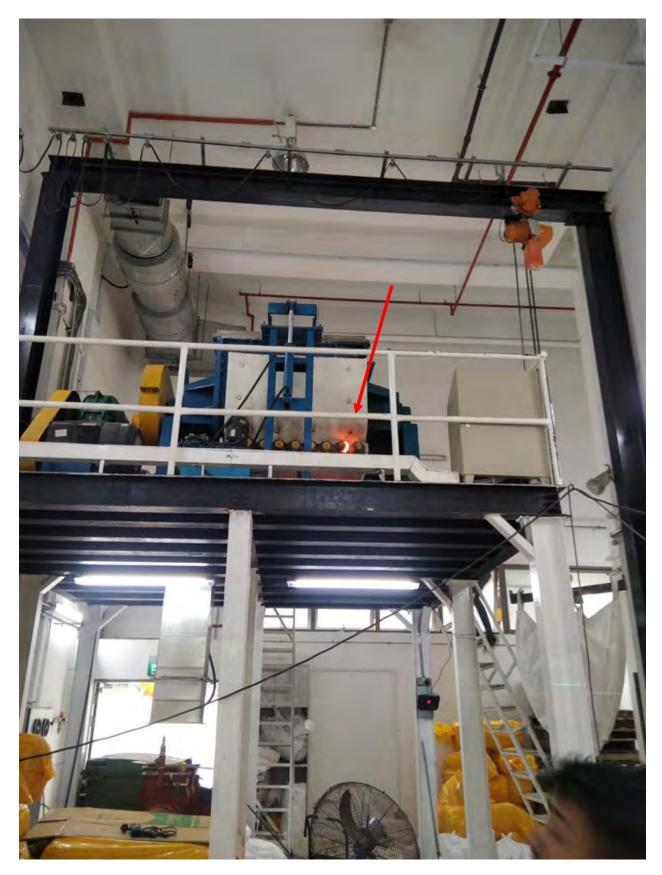
**Photograph 9:** Photograph sent to me by Mr Chua. The red arrow is pointing to the fire involving the machine. The fire is centred on the second heater from the right. The image shows that the thermal insulation of the machine is intact and below the mezzanine the surfaces appear free of dust.
