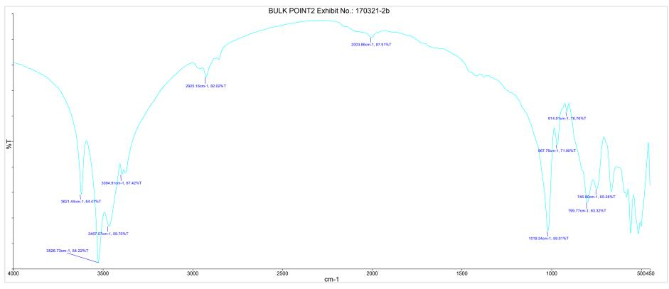
Figure 7 – FTIR spectrum of Specimen 7 - Bulk Point 2, Exhibit No. 170321-2b
