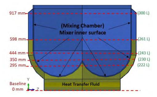
2 **Figure B.4.** Variation of heat transfer fluid volumes and their corresponding levels within the heating jacket.
