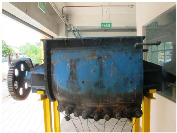
**Photograph 44:** The machine as seen at Matcor. Note the orange chalk marks indicate the intended cut-lines.
