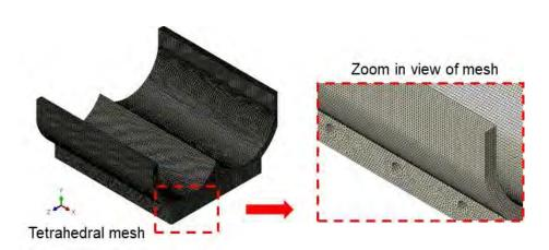
Figure B.2. FEA mesh for heat transfer fluid within the jacket
