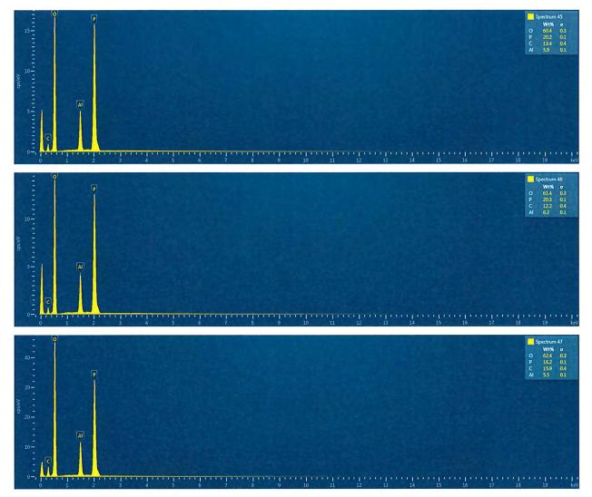
Figure 12c: EDX Spectrums 45 to 47 - Elemental Compositions of "Bulk (Aluminium Dihydrogen Phosphate), (170321-7b)"
