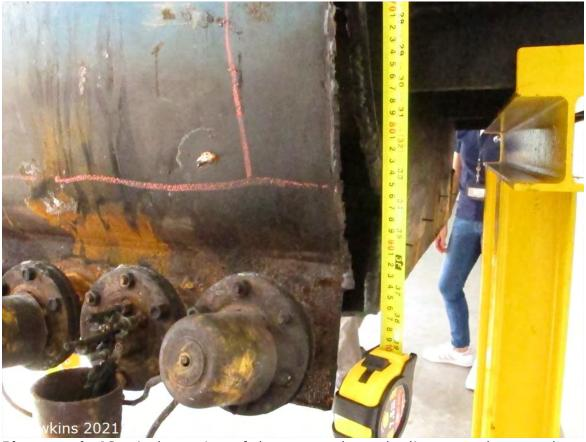
**Photograph 46:** A closer view of the tear at the end adjacent to the control panel. Note how the side wall of the oil reservoir had distorted outwards.
