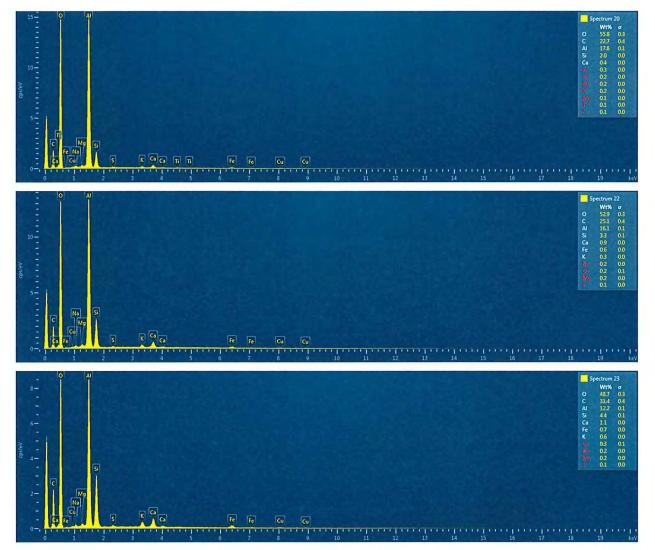
Figure 6c: EDX Spectrums 20, 22 and 23 - Elemental Compositions of "Bulk Point 1, (170321-1b)"
