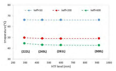
10 **Figure 6.** Maximum temperatures (average of HTF and mixer surface) obtained under high convective heat transfer conditions (h=500 W/m<sup>2</sup>K) with a 7.2 kW heating source input
