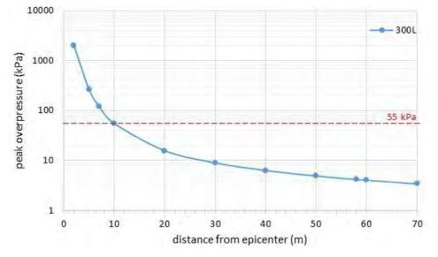
Figure 19. Graph of overpressure against distance for HTF volume = 300L
