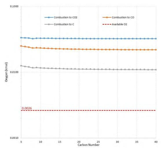
Figure 2. Plots of oxygen required for the complete and incomplete combustion of C5 to C40
