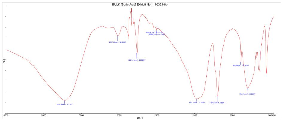
Figure 13 – FTIR spectrum of Specimen 13 - Bulk (Boric Acid), Exhibit No. 170321-8b
