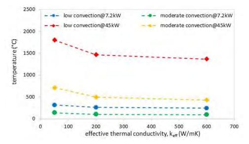
**Figure 9.** Effect of increased heat source power on the mixer's temperature profile **Note:** low convection,  $h = 5 \text{ W/m}^2\text{K}$  whilst moderate convection,  $h = 50 \text{ W/m}^2\text{K}$ .
