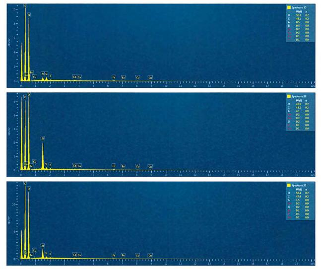
Figure 10c: EDX Spectrums 35, 36 and 37 - Elemental Compositions of "Bulk (Platform) 5, (170321-5b)"
