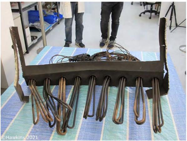
**Photograph 54:** The oil reservoir heating elements. The three elements on the left (this end had been closest to the control panel) had been bent in towards the centre of the reservoir.
