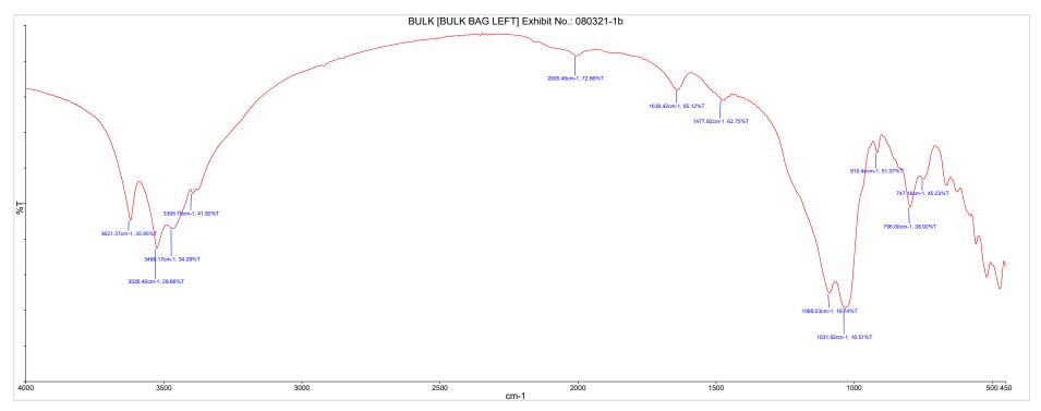
Figure 2 – FTIR spectrum of Specimen 2 - Bulk (Bulk Bag Left), Exhibit No. 080321-1b
