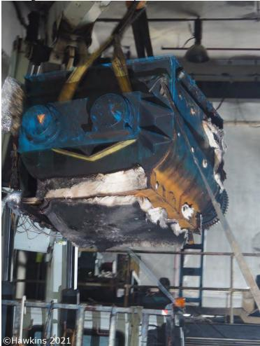
**Photograph 34:** The thermal insulation remained attached to one end and the underside of the machine.
