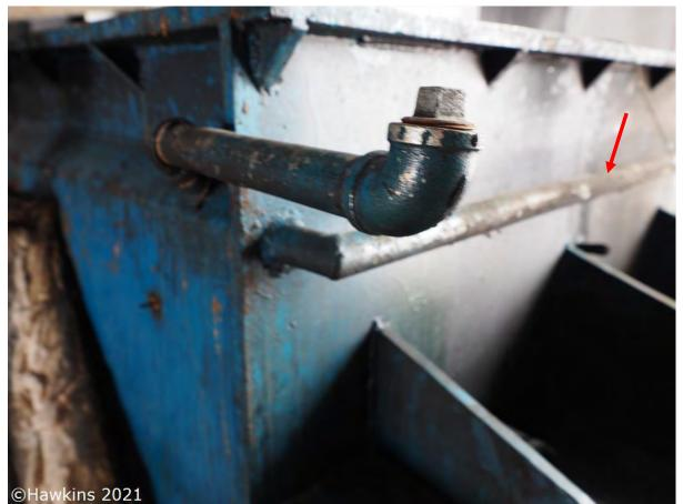
**Photograph 31:** One of the oil reservoir filling points. Note that it is capped. The pipe connecting the two halves of the reservoir is highlighted by the arrow.
