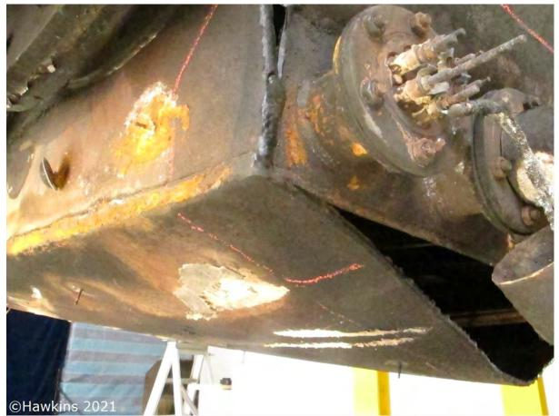
**Photograph 47:** The bottom of the oil reservoir was distorted downwards.
