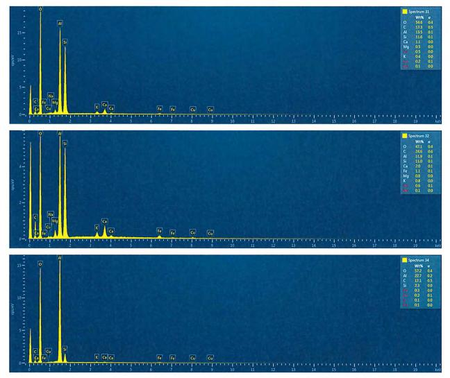
Figure 9c: EDX Spectrums 31, 32 and 34 - Elemental Compositions of "Bulk (Under Pallet) 4, (170321-4b)"
