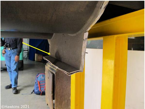
**Photograph 50:** The inside of the oil reservoir looking across the underside of the reaction vessel from the location of the corner closest to the control panel. What appears to be a 'spray' mark is apparent.
