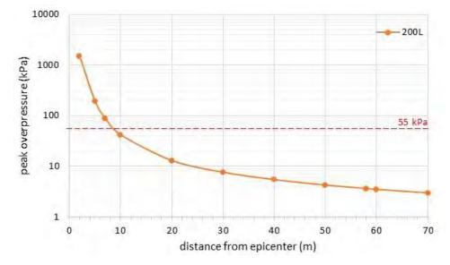
Figure 20. Graph of overpressure against distance for HTF volume = 200L
