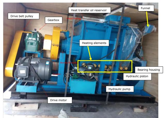
**Photograph 2:** The machine in its crate with key parts annotated. The locations of the filling funnel and heating elements are highlighted.
