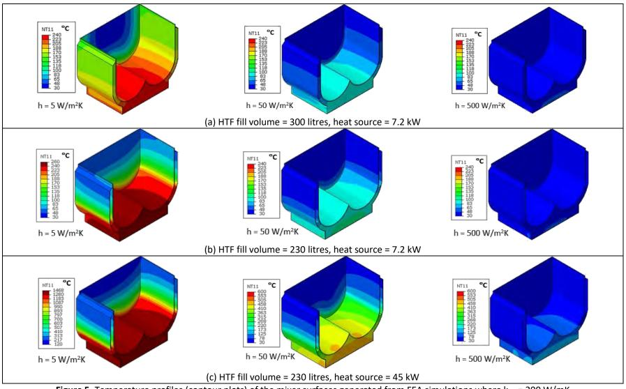
**Figure 5.** Temperature profiles (contour plots) of the mixer surfaces generated from FEA simulations where  $k_{eff} = 200 \text{ W/mK}$
