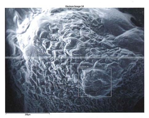
Figure 12b: SEM/EDX image of "Bulk (Aluminium Dihydrogen Phosphate), (170321-7b)"
