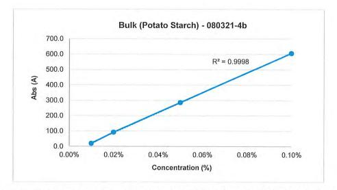
Figure 2 – Reference spectrum standard curve of Specimen 5 - Bulk (Potato Starch), Exhibit No. 080321-4b
