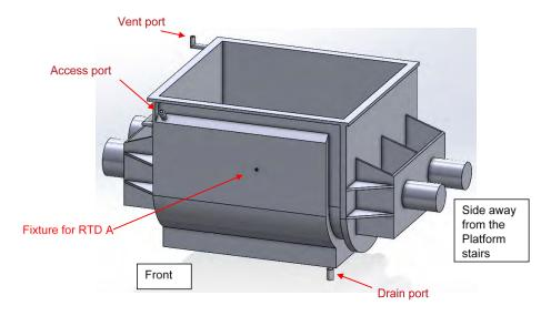
Fig. 1: Front view of Mixer Machine
