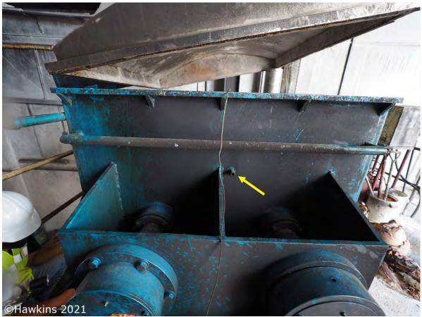
**Photograph 29:** What appeared to be a port for a second thermocouple. No thermocouple was in-situ.
