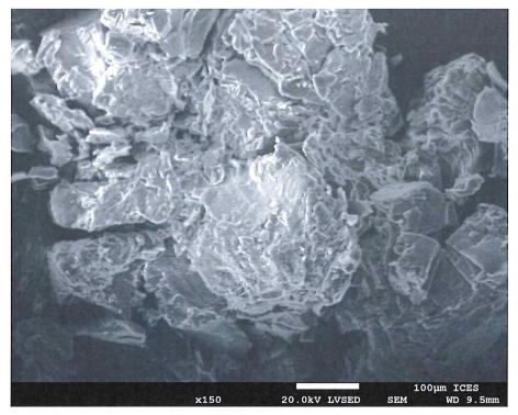
Figure 13a: SEM image of "Bulk (Boric Acid), (170321-8b)"
