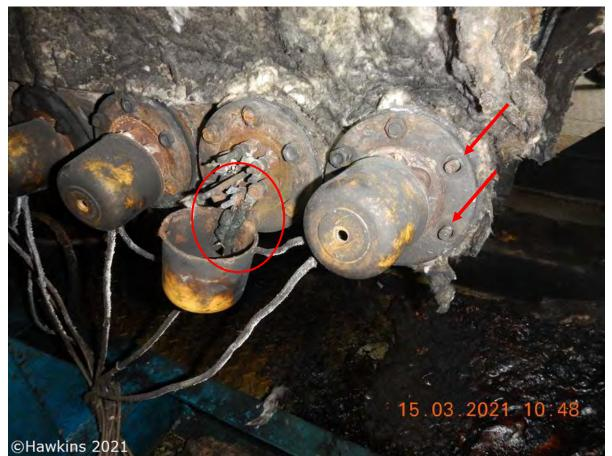
**Photograph 41:** The heads of the heating elements. Note the insulation tape wrapped around the cables of the element that had caught fire earlier in the day. Also note the two missing nuts (arrowed) of the heating element next to it (see Photograph 30).
