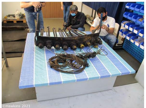
**Photograph 53:** The oil reservoir heating elements.
