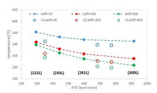
18 **Figure 8.** Maximum temperatures (average of HTF and mixer surface) obtained under low convective heat transfer conditions (h=5 W/m<sup>2</sup>K) with a 7.2 kW heating source input
