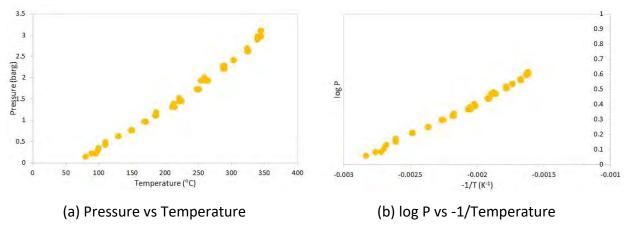
Figure E.3. Parr Reactor experimental Run 3 up to 340  $^\circ\text{C}$
