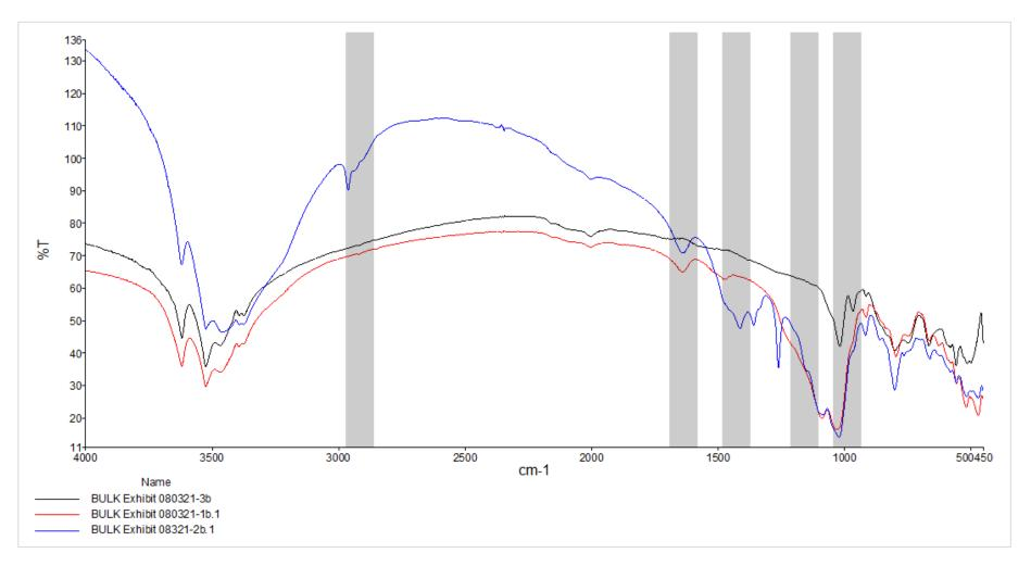
Figure 16b – FTIR spectrum comparison of Specimens 2, 3 and 4
