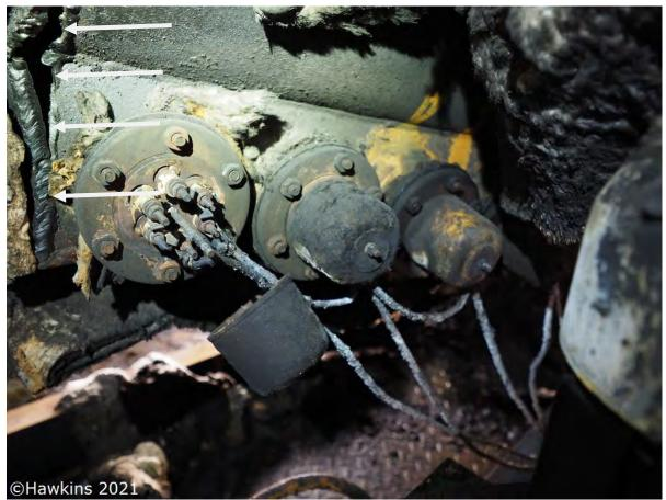
**Photograph 37:** The tear in the oil reservoir casing relative to the heating elements.
