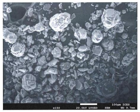
Figure 4a: SEM image of "Bulk (Aluminium Hydroxide), (080321-3b)"
