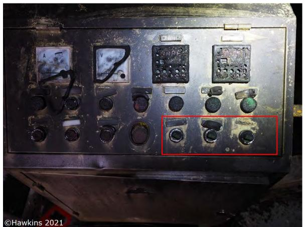
**Photograph 27:** The damage to the control panel. The heater switches are highlighted.
