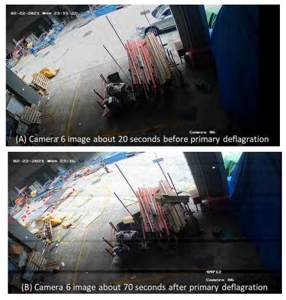
Figure 25. Images from CCTV Camera 6 showing the translation of large metal and cardbox sheets
