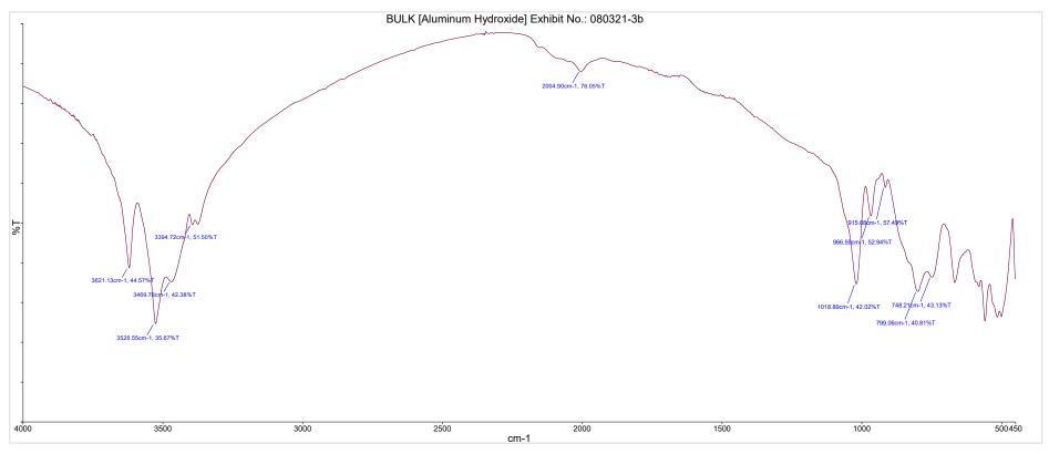
Figure 4 – FTIR spectrum of Specimen 4 - Bulk (Aluminium Hydroxide), Exhibit No. 080321-3b
