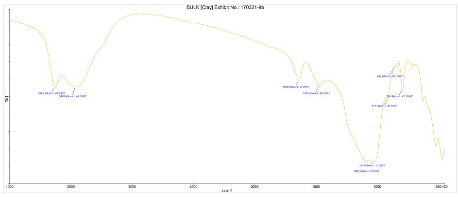
Figure 14 – FTIR spectrum of Specimen 14 - Bulk (Clay) Exhibit No. 170321-9b
