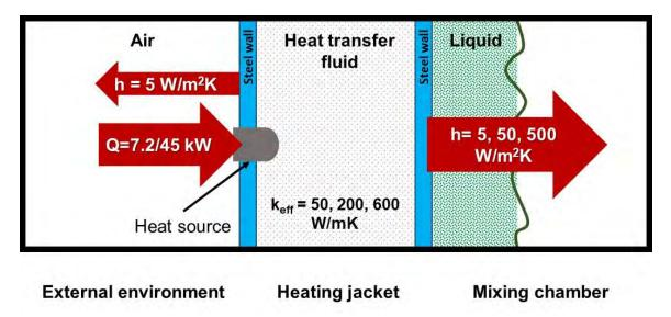
Figure 4. Overview of FEA heat transfer conditions for mixer
