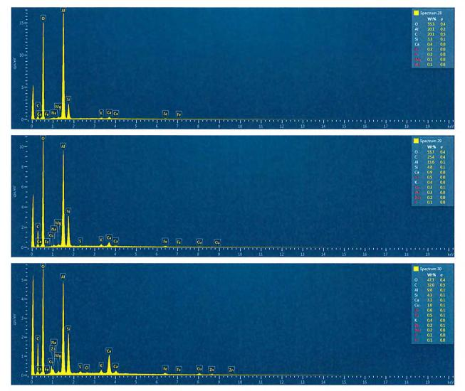
Figure 8c: EDX Spectrums 28 to 30 - Elemental Compositions of "Bulk Point 3, (170321-3b)"
