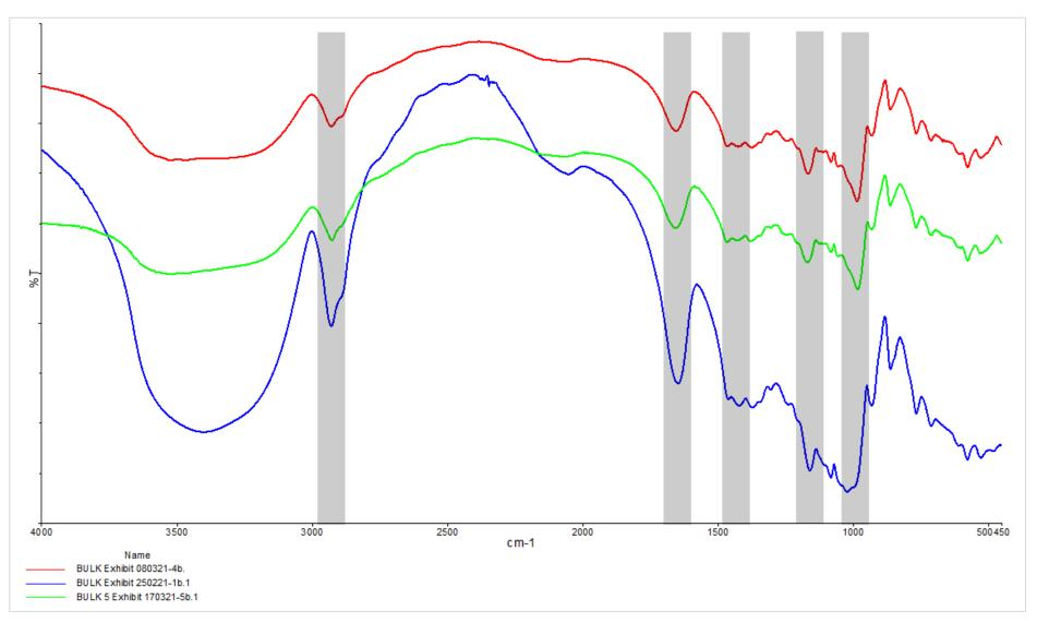
Figure 15 – FTIR spectrum comparison of Specimen 1, Specimen 5 and Specimen 10
