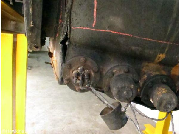
**Photograph 45:** A closer view of the tear at the drive-motor end. Note how the end wall of the oil reservoir had distorted outwards.
