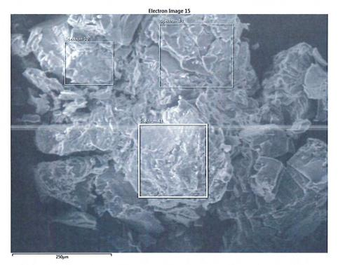
Figure 13b: SEM/EDX image of "Bulk (Boric Acid), (170321-8b)"
