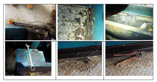
**Photograph 30:** Montage of the spare heater with a socket and ratchet (top left) and the selection of tools left on the machine and mezzanine. They included spanners, a screwdriver and cable crimps. Note the two nuts on the machine next to the spanners (bottom left image).
