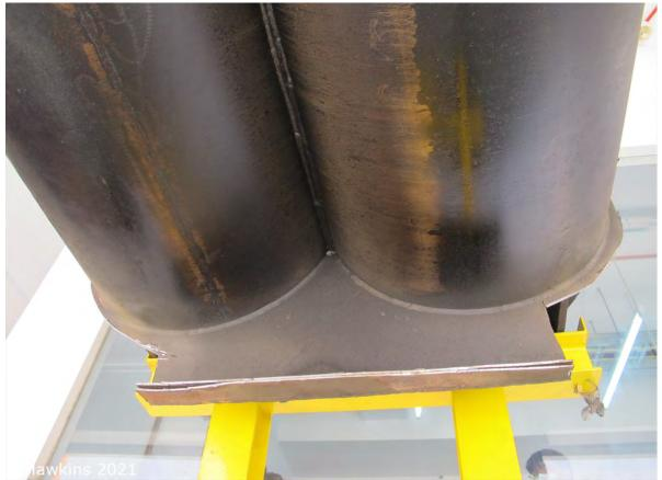
**Photograph 49:** Photograph 48 in context. Note there is no evidence of a tidemark on the end wall of the reservoir to indicate the oil level before the explosion.
