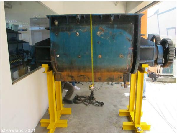
**Photograph 43:** The machine as seen at Matcor. Note the orange chalk marks indicate the intended cut-lines.
