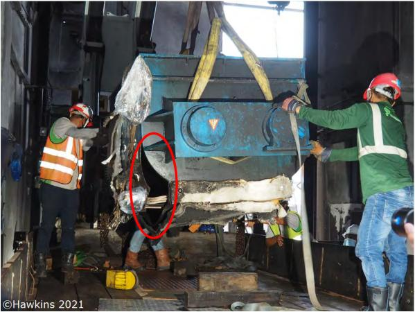
**Photograph 38:** The end of the machine that had been closest to the control panel. Note the insulation material is still in-situ and the tear in the oil reservoir casing by the heaters.
