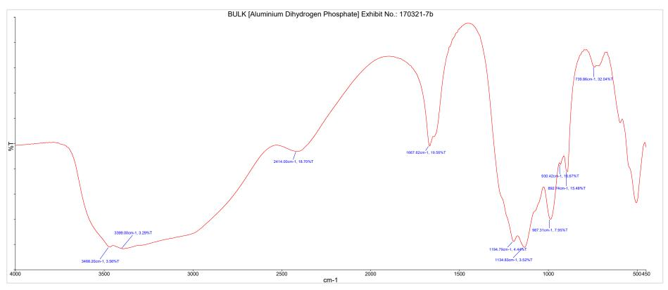
Figure 12 – FTIR spectrum of Specimen 12 - Bulk (Aluminium Dihydrogen Phosphate), Exhibit No. 170321-7b
