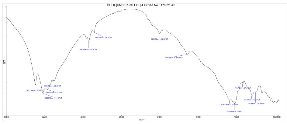
Figure 9 – FTIR spectrum of Specimen 9 - Bulk (Under Pallet) 4, Exhibit No. 170321-4b
