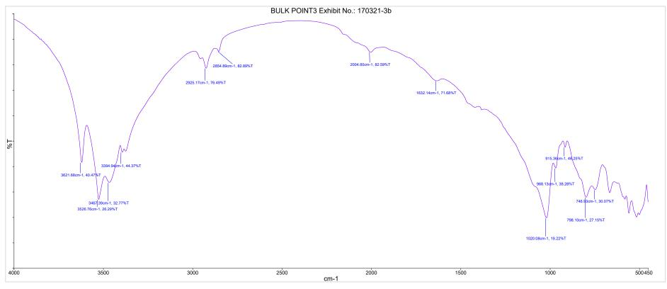
Figure 8 – FTIR spectrum of Specimen 8 - Bulk Point 3, Exhibit No. 170321-3b
