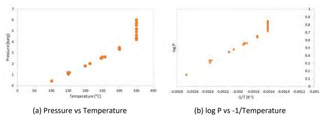
Figure E.5. Parr Reactor experimental Run 5 up to 350 °C
