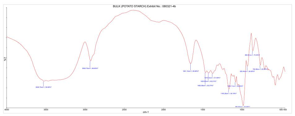
Figure 5 – FTIR spectrum of Specimen 5 - Bulk (Potato Starch), Exhibit No. 080321-4b
