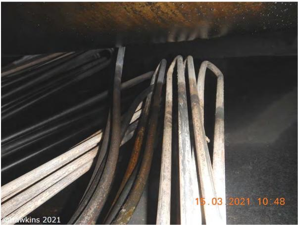
**Photograph 40:** The distortion of the heating elements closest to the control panel.
