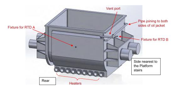
Fig. 2: Rear view of Mixer Machine
