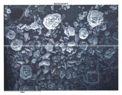
Figure 4b: SEM/EDX image of "Bulk (Aluminium Hydroxide), (080321-3b)"
