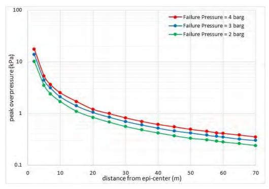
14 **Figure 16.** Graph of overpressure against distance for heating jacket failure at pressure P = 2, 3 and 4 barg
