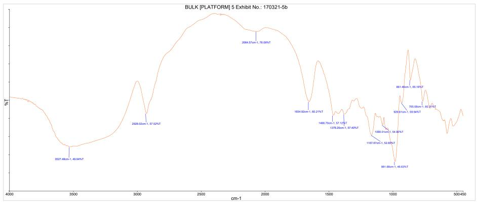
Figure 10 – FTIR spectrum of Specimen 10 - Bulk (Platform) 5, Exhibit No. 170321-5b
