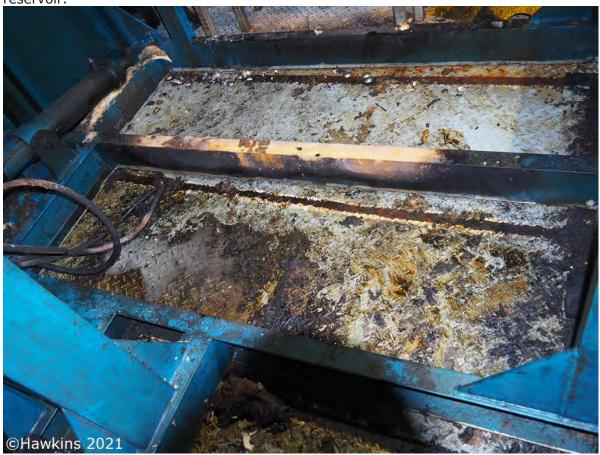
**Photograph 36:** The localised fire damage to the frame that supported the machine. The opposite side of the steel frame was hardly affected.
