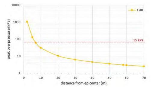
Figure 22. Graph of overpressure against distance for HTF volume = 120L
