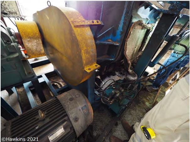
Photograph 33: The thermal insulation on the side of the machine fitted with the heating elements was mostly in-situ.
