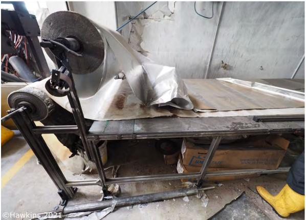
**Photograph 17:** Just inside the roller shutter looking away from electricity intake equipment. The items are heat damaged. Note the unburnt cardboard.
