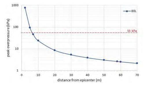
Figure 23. Graph of overpressure against distance for HTF volume = 80L
