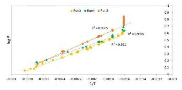
2 **Figure 13.** Consolidated graph of pressure logarithm against reciprocal temperature for experimental Runs 3, 4 and 5
