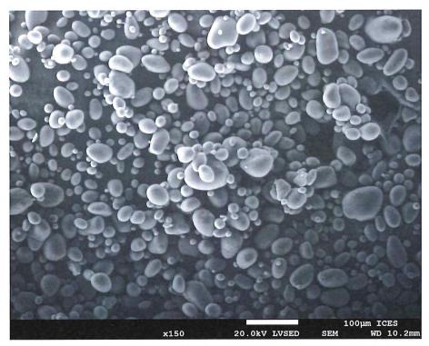
Figure 5a: SEM image of "Bulk (Potato Starch), (080321-4b)"
