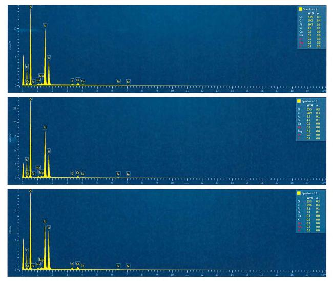
Figure 3c: EDX Spectrums 9, 10 and 12 - Elemental Compositions of "Bulk (Bulk Bag Right), (080321-2b)"
