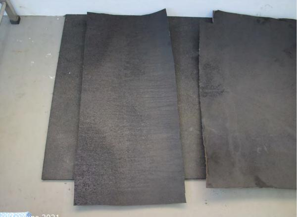
**Photograph 52:** The bottom and one side of the oil reservoir. Note the soot marks.
