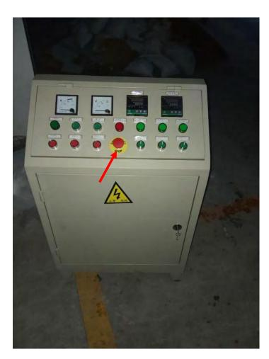
**Photograph 5:** The control panel of the machine incorporated an emergency stop button (arrowed).
