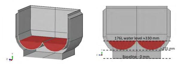
Figure 10. Illustration of mixing chamber with a water fill of 176 litres of water
