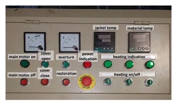
Fig. 3: Photograph of the control panel, with labels added (obtained from MOM)
