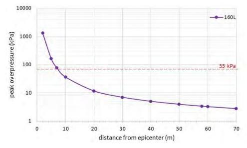
Figure 21. Graph of overpressure against distance for HTF volume = 160L
