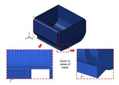
Figure B.1. FEA mesh for mixer structure
