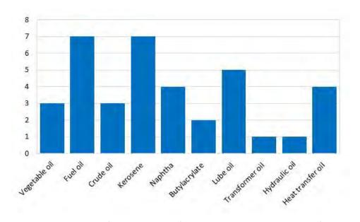
Figure 17. Breakdown of aerosol related fires and explosions according to fuel type
