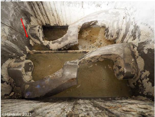
**Photograph 28:** The mixing chamber of the machine. The thermocouple wire is highlighted.
