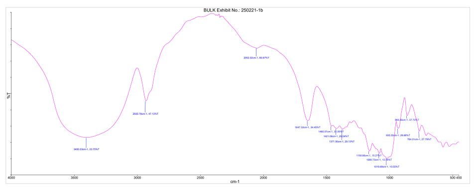
Figure 1 – FTIR spectrum of Specimen 1 - Bulk, Exhibit No. 250221-1b
