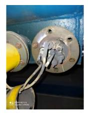
(2) Photo of damaged Heater No. 1, sent by Imam to Mr Chua on 8 August 2020,9:40am [S-6]:
