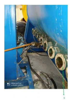
49. The old worn-out gaskets were replaced by new gaskets.
