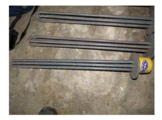
22. The metal tubes portion of the heaters would be inserted into the bottom of the oil jacket through openings for the heaters. There were gaskets placed between the openings and the heater flanges. From the outside, the flanges would be bolted to the openings, to keep the heaters in place. Yellow hub caps covered the heater terminals **[S-59]**.
