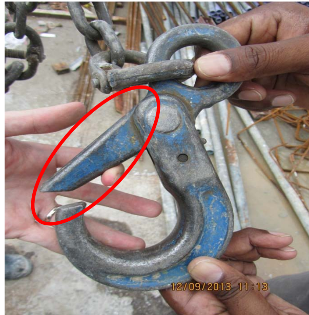
Figure 7b A defective safety hook latch of a lifting gear which is ineffective in retaining slings or other lifting devices.
