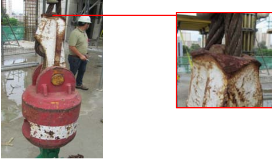
Figure 4 A badly corroded wedge socket used to terminate the wire rope. Corrosion can lead to early failure of crane components.
