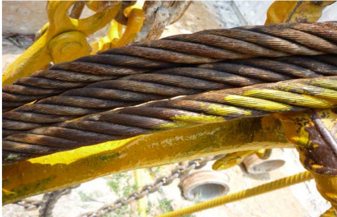
Figure 10 - Badly Corroded Lifting Gear due to lack of upkeep
