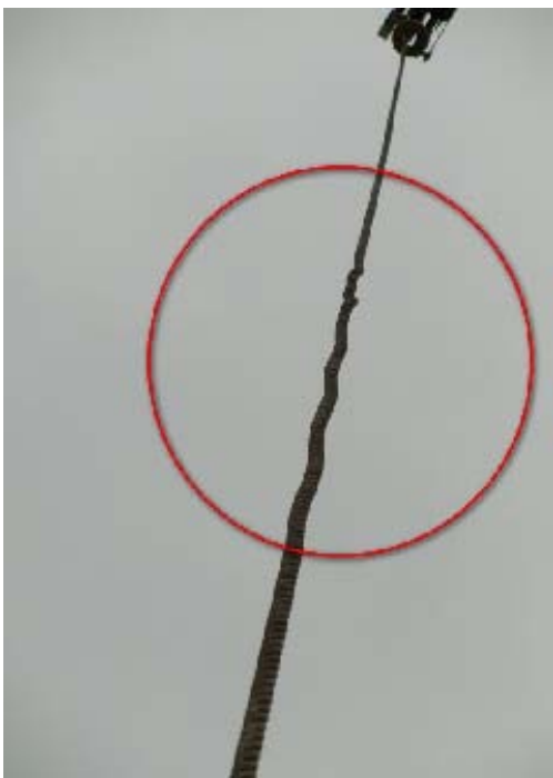
Figure 3 - Kinked main hoist Wire Rope
