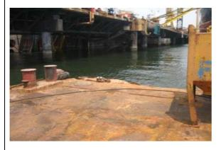
Failed to cover or guard openings through which a person might fall more than 2 metres by installing effective guardrails, barriers or other equally effective means to prevent fall,.
