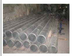
Failure to implement safe work procedures to control risk arising from the stacking, lifting and transferring of galvanised pipes.
