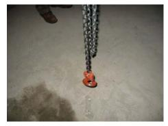
Failure to ensure every lifting appliance was marked conspicuously with its safe working load and a distinctive number or any other means of identification.
