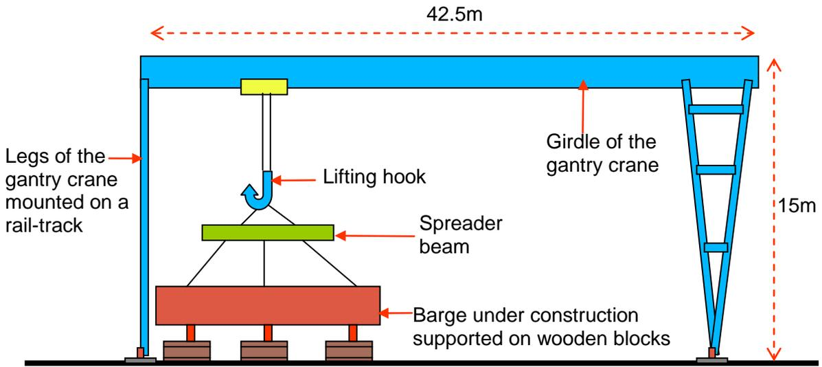
**Schematic of the gantry crane prior to accident**
