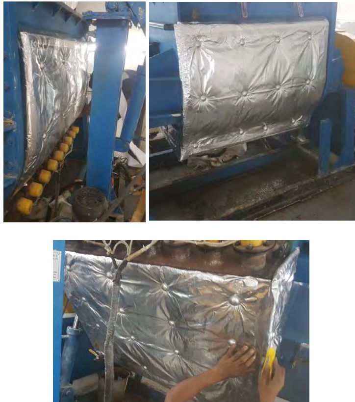
S-55: Photographs of the insulation on the oil jacket taken by Marimuthu on 6 February 2021
