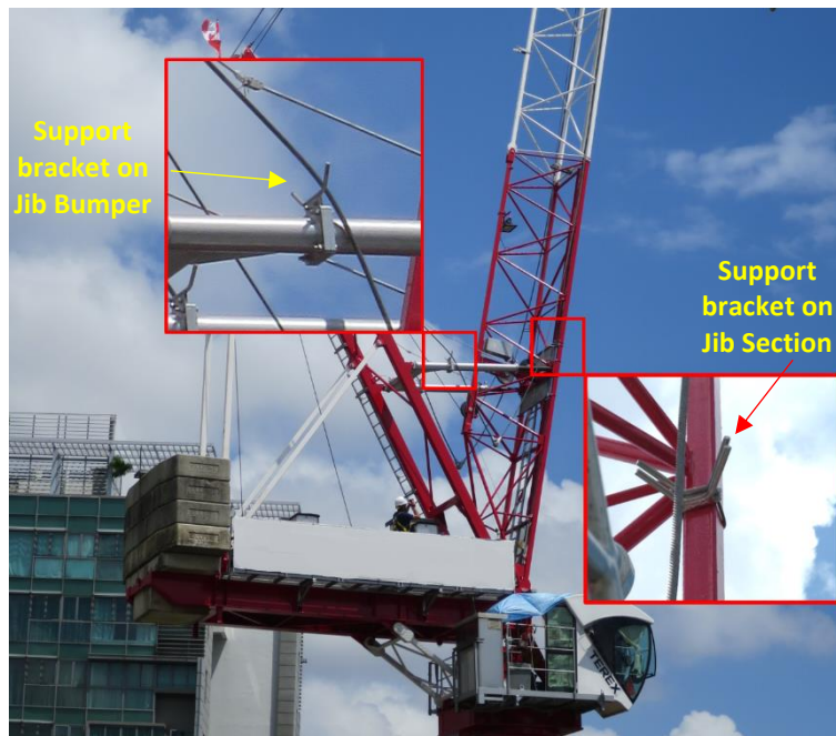
Figure 6 - Erection Ropes rest in the support bracket when the jib is raised
