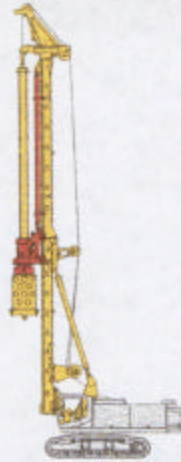
Hydraulic Boring rig for Bored Pile and Secant Pile
