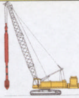
Deep Vibrator Rig for Soil Improvement at Reclamation work
