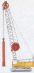
Grab Rig for Diaphragm Wall Construction.
