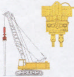
Top Vibrator Rig for Sheet Pile and install Temporary Casing
