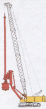
Mechanical Boring Rig for Bored Pile
