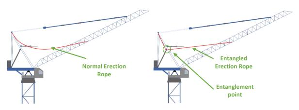
Figure 8 - Schematic views of the TC showing conditions with normal and entangled Erection Rope
