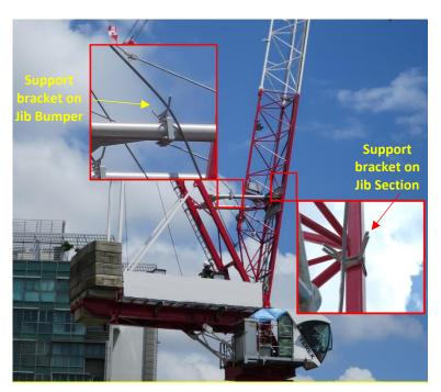
Figure 6 - Erection Ropes rest in the support bracket when the jib is raised
