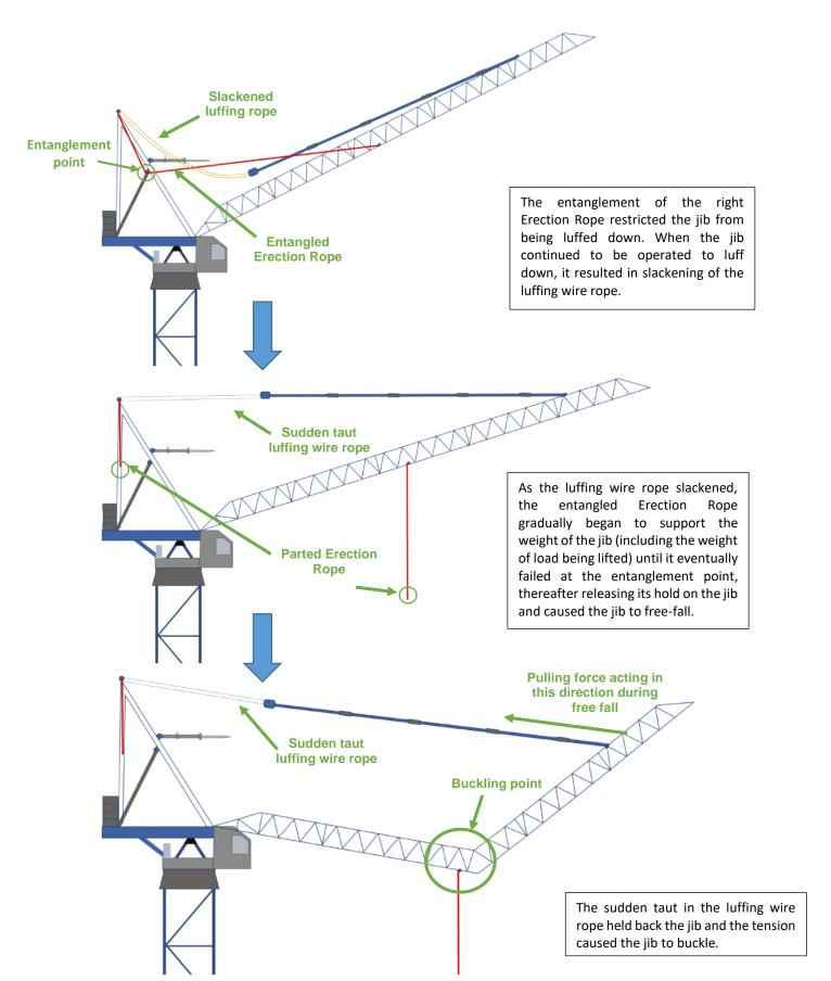
Figure 9 – Sequence of events on the buckling of luffing jib of the TC
