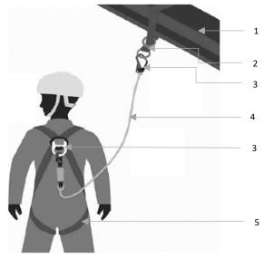
Components of a personal fall arrest system are shown below:
